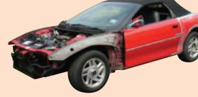
It's takes 3-4 hours to remove the Camaro hood, bumper, fenders, taillights, rear bumper cover and gas cap door. Our fiberglass components bolt on, screw on and glue on in approximately 50 man hours.
