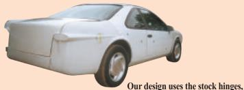
latch, solenoid, and weather strip ensuring a much better seal than any custom built set-up. Also the 1/4 panel skin overlays fit into the original trunk gap and wheel lip. They start over the wheel area about as thick as a pizza box & get thicker as they go back. As a result, very little blending is required.
