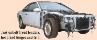
front radiator support. This is the only cutting on the car! The radiator, battery and all mechanicals stay in place. The only thing disconnected are the lights. The car stays fully mobile.
