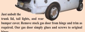
adhesive THIS IS THE BEAUTY upper lip PART OF THE DESIGN! inner lip When these cars are built by custom builders, the entire rear section is cut off both the 49-51 & 89-97 models and modified to fit. Our patent pending design ELIMINATES ALL THE CUTTING, WELDING, & HARD WORK. The upper lip goes into the original trunk gap and the inner lip surrounding the wheel area simply glues and screws to the 89-97 vehicle 1/4 panel.
